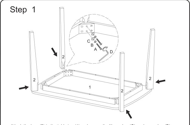
Attach the legs (2) to the table top (1) and secure it with washer (C), spring washer (B), bolt (A) and wrench (D).
