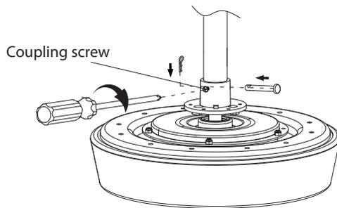
Slide downrod into the coupling on top of the motor. Install the hanging pin by aligning the holes in the coupling with holes in the downrod. Secure hanging pin with locking pin. Securely tighten the two previously loosed set screws.
