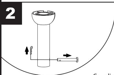
Loosen the two coupling screws preassembled in the coupling, but do not remove them. Remove the locking pin and hanging pin from the downrod assembly. Retain for later use.
