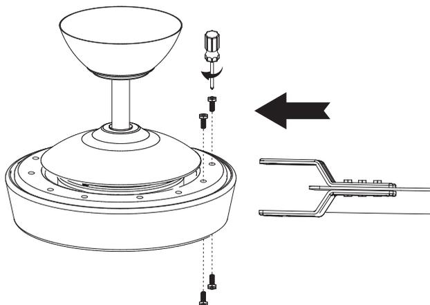
Position blade assembly along the motor and make sure the blade arm is fully seated against the flywheel. Tighten them with four blade screws.
