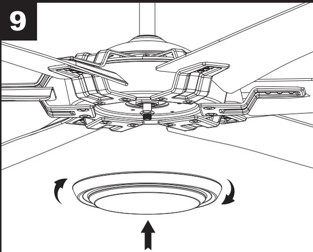
Assemble the cap to the threaded rod by twisting in a clockwise direction.
