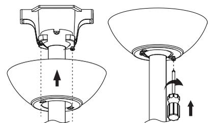
Loosen the screws without fully removing it. Assemble canopy by rotating key slot in canopy over screws in mounting bracket, taking care not to pinch the wires. Tighten the screws.
