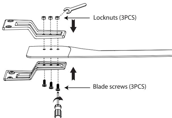
Attach blade arms to blade as shown. Screw the blade screws (provided in the hardware bag) into the screw holes and tighten it with the locknuts by using a wrench.
