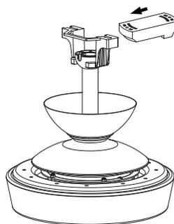
Slide the receiver into the open end of the mounting bracket with the flat side of the receiver facing the ceiling.
