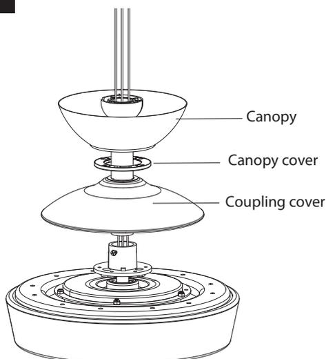
Place downrod assembly through canopy, canopy cover and coupling cover. Route the motor lead wires through the downrod assembly.
