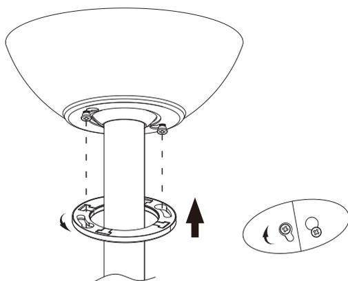
Securely attach and tighten the canopy cover over the screws in the mounting bracket utilizing the key slot twist-lock feature.
