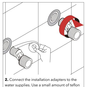
tape to ensure a watertight seal.
