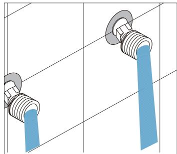
**4.** Turn the water on for several minutes to flush the supply lines. This will prevent dirt and impurities from entering the cartridge and reducing water pressure.
