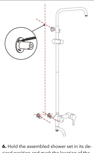
**6.** Hold the assembled shower set in its desired position and mark the location of the mounting bracket.
