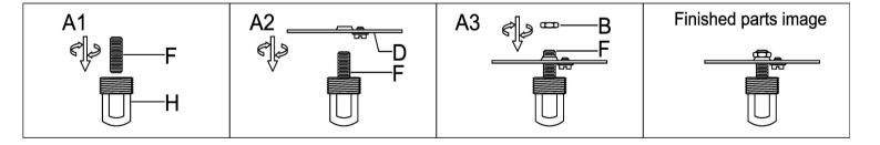
Step A1:Fix the threaded nipple(F) into the screw collar loop(H)
