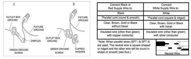
Twist plastic wire connector(A) until wires are tightly joined together, wrap each connector
