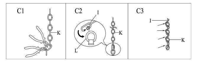
Step C1: By measuring, determine the correct length of links needed. Use the chain pliers,
