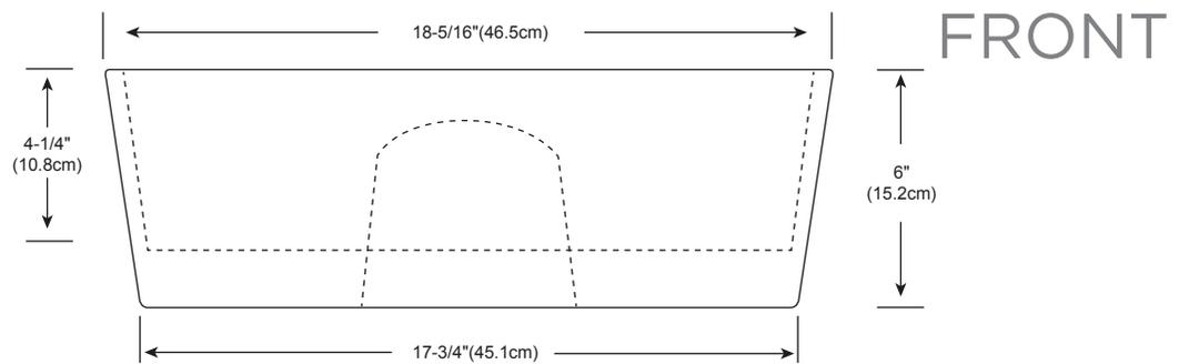
By IAPMO, ceramic lavatory warpage is defective only if warpage of flat slab out of horizontal plane exceeds 6.3 mm/m (0.25 in/ft) on all sizes OR warpage on back of lavatories that are attached to the wall exceeds 3 mm (0.13 in).
