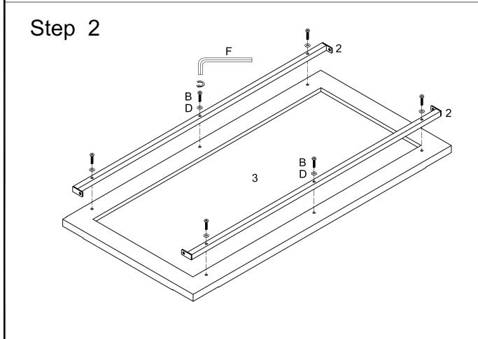
Attach part (2) to part (3) using bolts (B) and washers (D) as shown.
