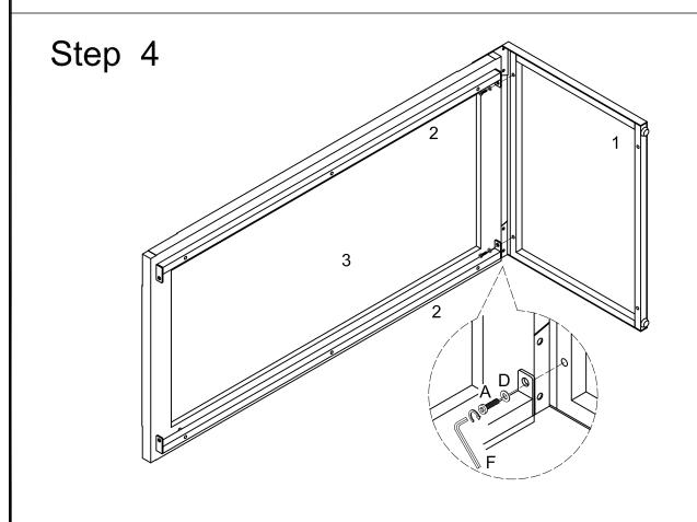
Join top panel (3) to part (1) using bolts (A) and washers (D).
