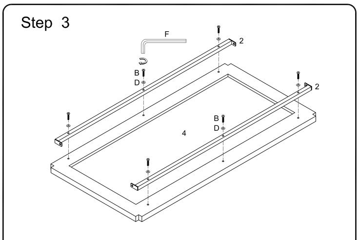
Attach part (2) to part (4) using bolts (B) and washers (D) as shown.
