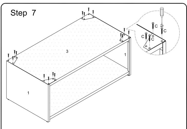
Secure top panel (3) at the metal caps using screws (C) as shown in the diagram
