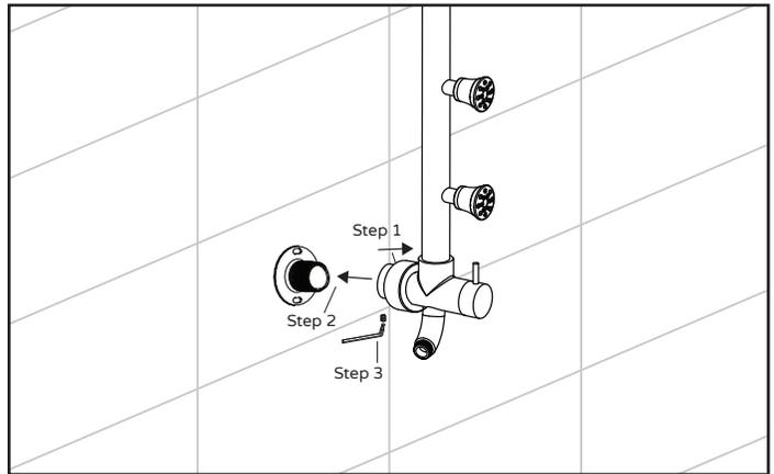
Step 1: Slide escutcheon (6) back in order to place set screw (4) later on.
