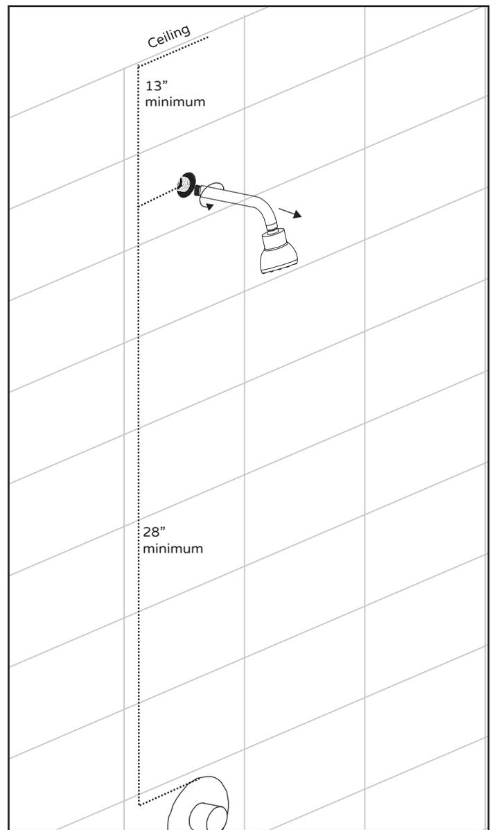
Remove existing shower arm and shower head. Make sure distance from water outlet and mixing valve trim (NOT INCLUDED) is a minimum 28" or more.
