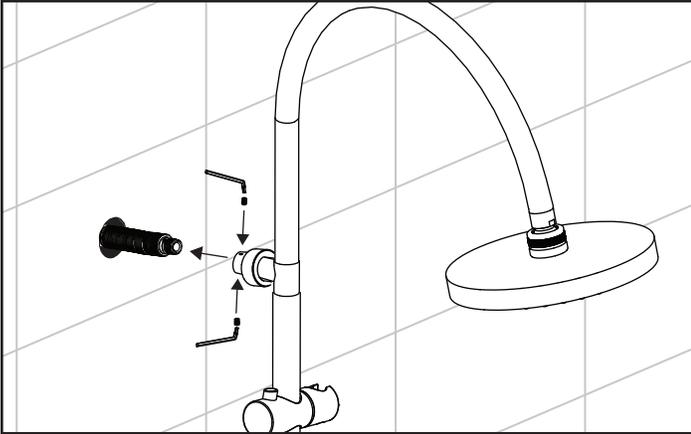
Attach assembled shower to inlet nipple (8) and secure set screws (4) with allen wrench (24) provided.
