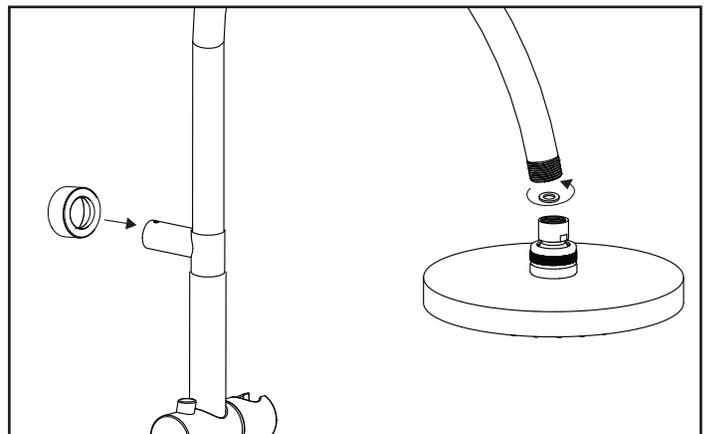
Slide escutcheon (6), insert washer (26), and screw showerhead (1) to shower arm (2) and secure.
