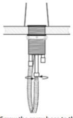
3. Screw the spray hose to the spray hose pipe.
