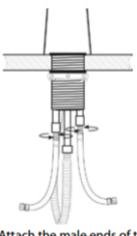
4. Attach the male ends of the flexable hoses to the hot and cold brass pipes on the faucet
