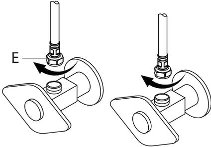
Attach waterlines (E) to angle stops and tighten until snug. Turn on angle stops and check for leaks (DO NOT TURN FAUCET ON).
