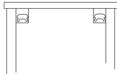
**STEP 3:** Install mounting plates (2) to the wall with provided hardware. Use proper hollow wall anchors if necessary. (Not provided)
