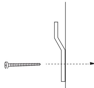
**STEP 4:** Install cabinet to wall. Insuring mounting brackets catch mounting plates.
