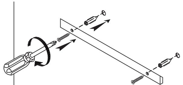
**IMPORTANT:** Consult an expert for the proper screws/bolts to use when attaching to various constructions. Screws provided do not attach to all wall construction types. Anchors are not required if brackets are installed in stud.
