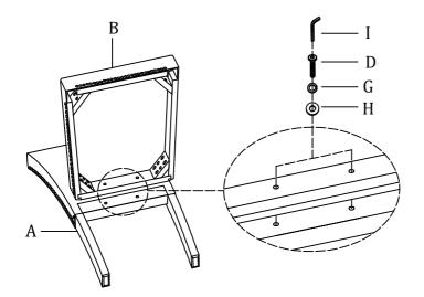
Take the Allen Wrench, and turn the bolts until the legs are secured. DO NOT TIGHTEN COMPLETELY. Stop when you feel you are adding force to tighten the bolt.
