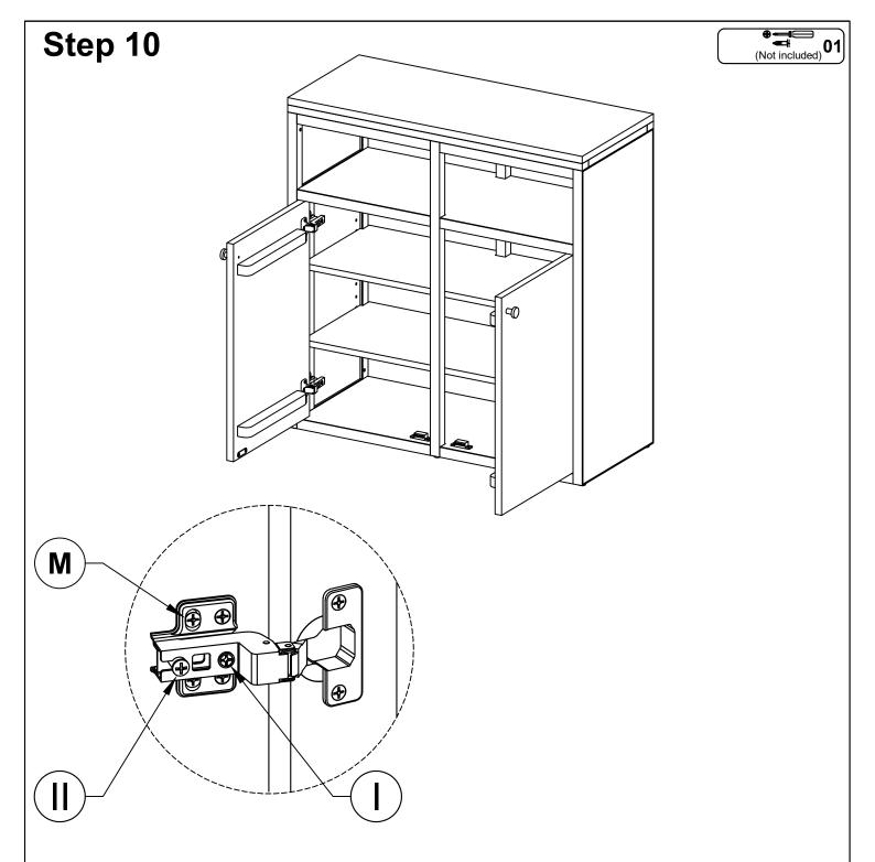
Tighten the Screw marked (II) to fasten hinge. The door may need to be adjusted so that all the spaces between the door and the unit sides are equal. To adjust, follow instructions:
