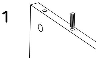
Put in the dowel inside the indicated hole and softly hit it until it's fully inside.
