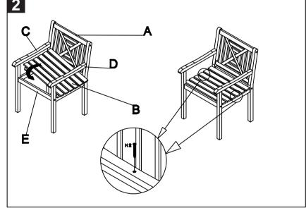
Step 1: attach left side (D) to the back (A). Then attach the supports (E) as shown on the picture by using the Allen Bolt (H1) and tighten it with the Allen Key (H4). Continue with the right side (C) in the same way. Make sure to tighten all bolts (H1) before you continue with step 2.
