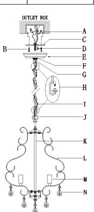
Step A1: Slip the loop (J) along wires then thread onto the nipple of top stem (K) till snug . Step A2: Adjust arms (L) to proper position.
