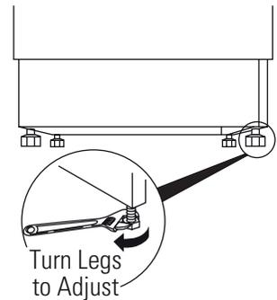
**TIP:** Pull lower rack out, about halfway. Check to be sure the rack does not roll forward or back into dishwasher. If the rack rolls in either direction, the dishwasher must be leveled again.
