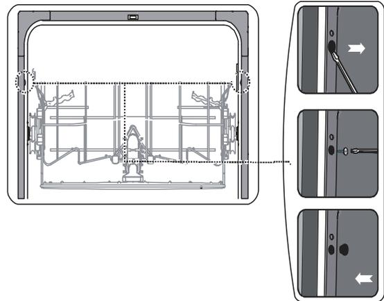
**IMPORTANT** – Drive screws straight and flush. Protruding screw heads will scratch the top of the control panel and can interfere with door closing.
