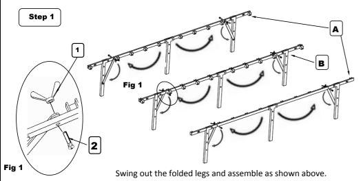
Use Bolt # 2 and Wing Nut # 1 to attach the support bracket to the side rail , See Fig 1  $\,$
