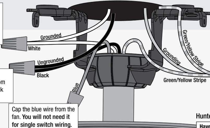
Connect the black (ungrounded) wire from the ceiling to the black wire from the fan.
