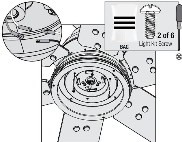
Partially install two of the light kit screws found in the hardware bag. It does not matter which two screw holes you choose. Connect the plugs from the upper switch housing and the LED assembly. Make sure to line up the colored markings on the connectors.
