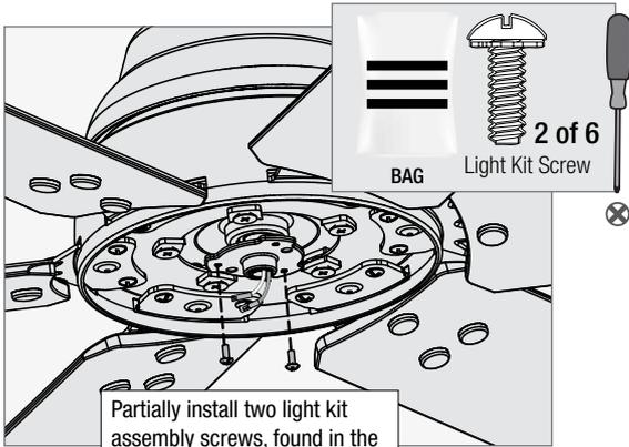
Partially install two light kit assembly screws, found in the hardware bag, halfway into the motor housing as shown. It does not matter which two screw holes you choose.
