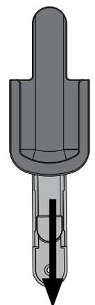
Slide the cradle onto the mounted bracket.
