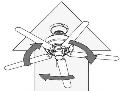
Updraft (clockwise rotation) creates a more indirect airflow. Updraft airflow is great for moving warm air downward.
