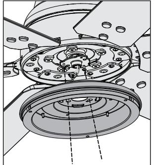
Feed the wire plugs through the center hole of the upper switch housing, then wrap keyhole slots around the screws and twist counterclockwise.
