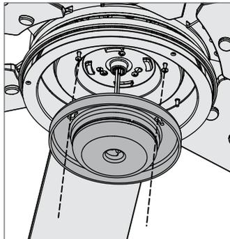
Align the keyhole slots in the light kit housing with the two screws. Make sure all the wires from the fan and the light kit are snug inside the center of the light kit, not pinched in between the upper switch housing and the light kit or hanging out of the sides.
