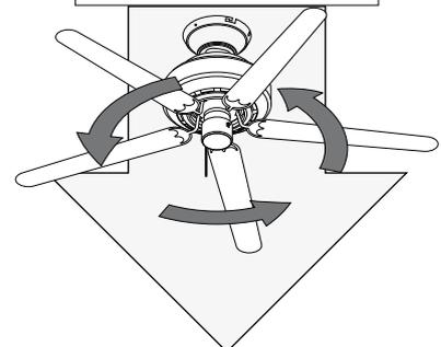
Downdraft (counterclockwise rotation) creates a direct breeze and maximum cooling effect.
