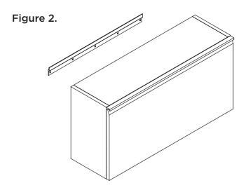
**Step 3:** Carefully lift and place the cabinet on the wall cleat.
