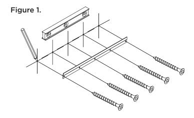
Step 2: Secure the wall cleat to the wall using the long screws provided.
