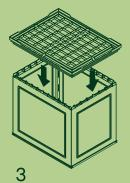
Flip the assembled body upright, tabs facing up. Then place the base, notches facing down, covering the opening.
