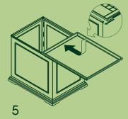
To attach the tray, rest the first few inches on top of the body, facing the arrow towards the opening. Then smoothly slide the tray forward until the opening is completely closed.
