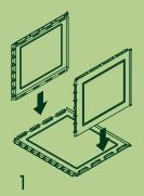
Click the short panels into the long panel by aligning the notches with the tabs.
