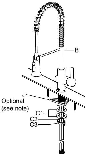
Install the plastic washer and metal washer (C1) onto the threaded mounting shank. Thread the nut (C2) onto the mounting shank. Lock the nut (C2) into position by tightening the screws (C3). Do not overtighten.
