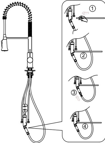
Connect the 1/4 in. water line from the filtration system by pushing the line into the connector (G). Pull down on the 1/4 in. line slightly to ensure the quick connect fitting has engaged.
