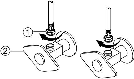
Thread the nut (1) on the supply line onto the outlet of the water supply valve (2) and tighten with wrench. Do not overtighten.
