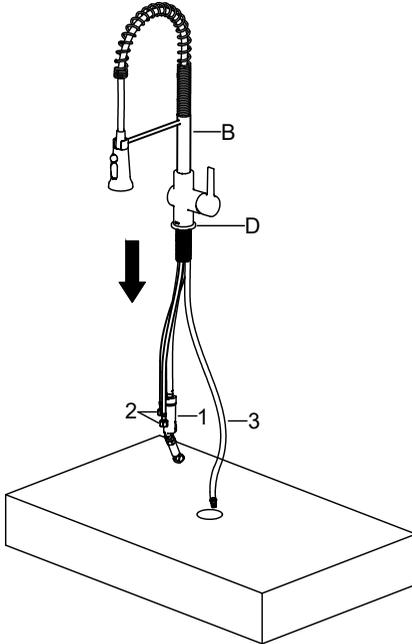
Before installation, ensure that the flange (D) is placed on the bottom of the new faucet assembly (B). Insert the faucet body and all hoses through the hole in the sink.
