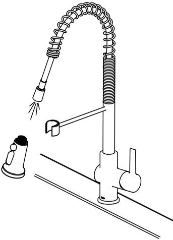
Pull hose assembly out of spout and remove spray head by unscrewing from hose in a counterclockwise direction. Hold the end of the hose down into the sink and turn the faucet on to the warm position. Flush water lines for one minute to flush away any debris. Check for leaks.
