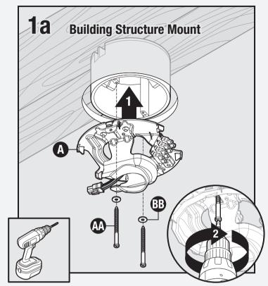
Using wood screws (**AA**) and washers (**BB**) included, install canopy mount (**A**) through box outlet into building structure. Drilling 9/64" pilot holes in building structure will aid in securing canopy mount (**A**).
