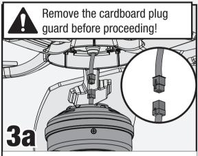
Connect the plugs from the fan and light fixture. Make sure to line up the colored markings on the connectors.
