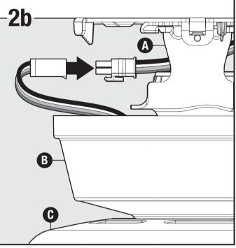
Connect wiring harness from canopy mount (A) to wiring harness from fan body (C).
