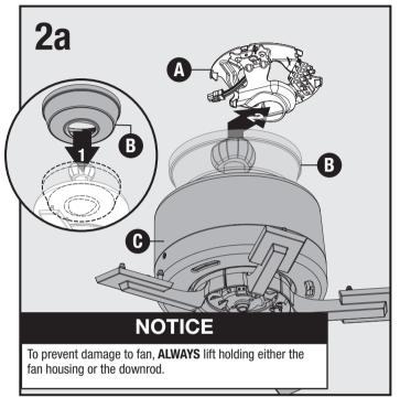
Install snap-on canopy (B) over downrod on fan body (C). Place the down rod ball into the slot in canopy mount (A) with built-in ceiling bracket.
