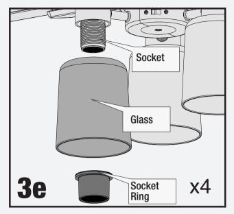
Remove the socket rings from the sockets. Install the glass onto the sockets. Install the socket rings onto the sockets. Tighten them by turning clockwise by hand.
