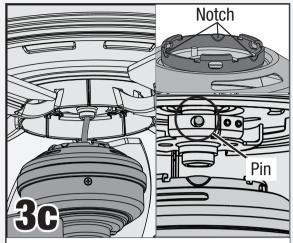
Raise the light kit to the bottom of the fan. Align the notch on the mounting ring on the top of the light kit with the pin in the mounting bracket on the bottom of the fan.
