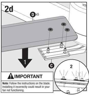
Install a snap-on blade to pop locks on pre-installed blade iron (C). Repeat for remaining blades (D).
