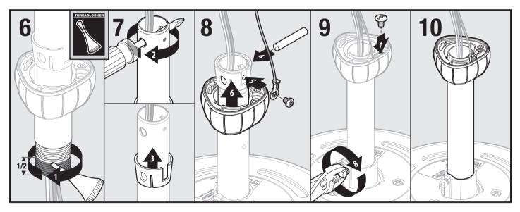
6. After cleaning pipe thread area, apply 1 ml threadlocker to lower half of downrod (1).
