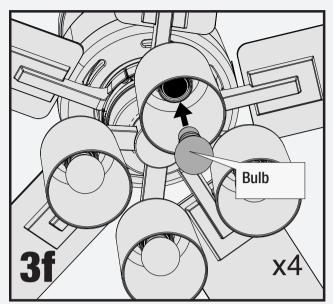
Install a bulb into each of the sockets. When necessary, replace with bulbs of same wattage.
