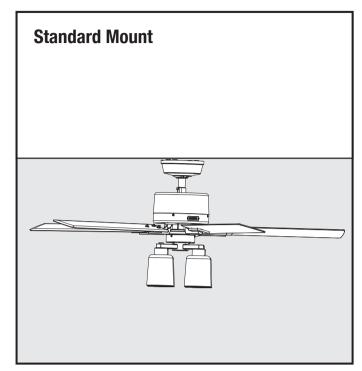
This installation is for **flat ceilings** using the short pre-installed downrod ceiling fans.
