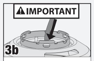
Push the connector and excess wire into the hole at the top of the light fixture. The connector and excess wiring must be pushed into the light fixture in order to successfully mount the light fixture to the fan.
