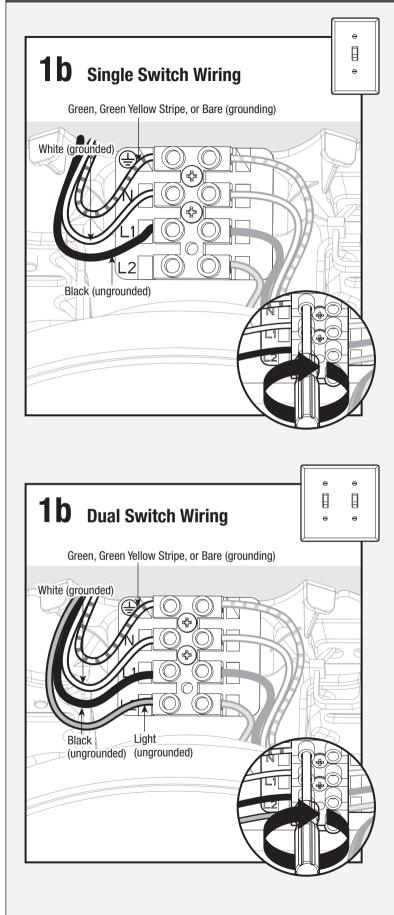
Connect wiring from ceiling to terminal block (on side of canopy mount) and tighten using flathead screwdriver (included).
