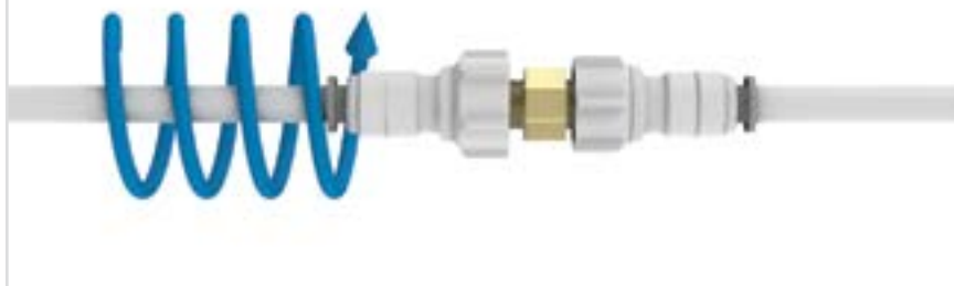
Diagram 2.6.4-A - Extending Quick Connect Tubing With Brass Compression Union
