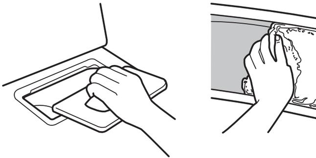
Clean the lint screen before each load. Pull the lint screen out of its holder. Roll lint off the screen with your fingers. Do not rinse or wash screen to remove lint. Push the lint screen firmly back into place. For additional cleaning information, see "Dryer Care".
