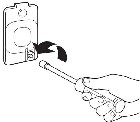
3. Turn bulb counterclockwise. Replace the bulb with a 10-watt appliance bulb only. Replace the cover and secure with the screw.
