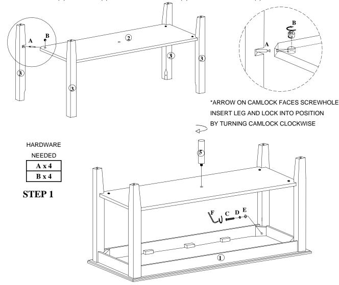
2. PLACE LEG ASSEMBLY ONTO TOP (1) AND FASTEN WITH ALLEN SCREWS (C) AND WASHERS (D) AND (E).
