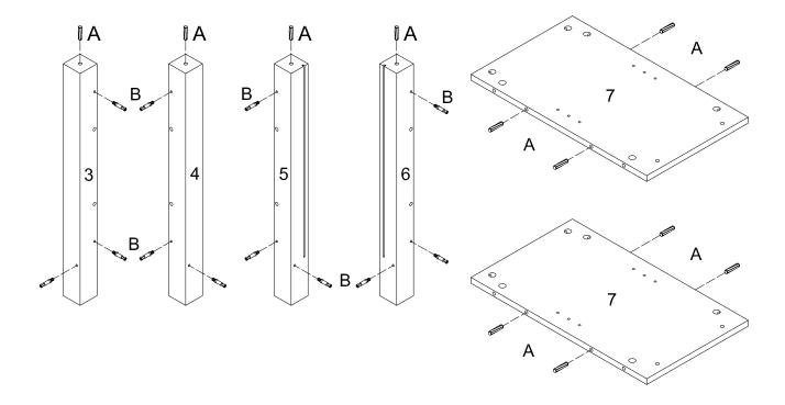
Insert wooden dowels (A) into designated areas in parts (3, 4, 5, 6) and (7). Attach cam bolts (B) to parts (3, 4, 5, 6).
