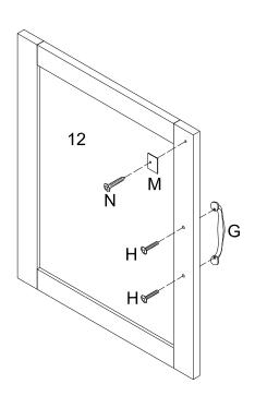
Attach handles (G) to the doors (11,12) by using screws (H). Attach metal stopper (M) using screw (N).
