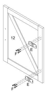
Attach hinges (E) to the doors (11,12) by using screws (F).
