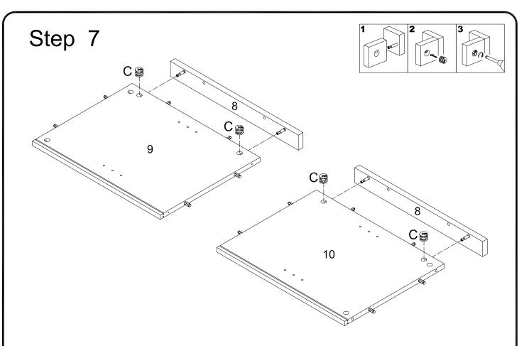
Attach cam locks (C) to part (9) to connect part (8), and to part (10) to connect to the other part (8).
