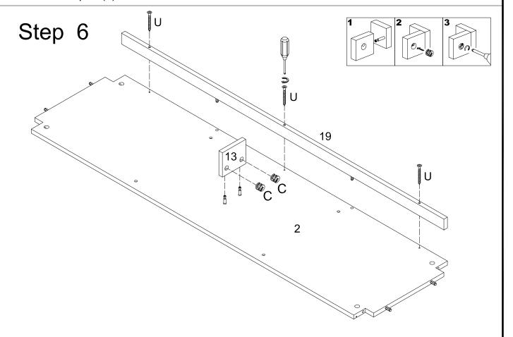
Attach cam locks (C) to parts (13) to panel (2). Attach slat (19) to panel (2) by using screw (U) as guides.
