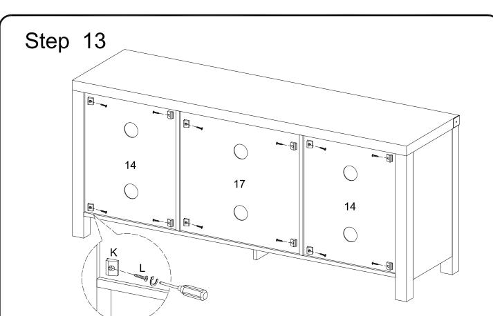
Attach the plastic wedges (K) by using the screws (L) as shown in the diagram.
