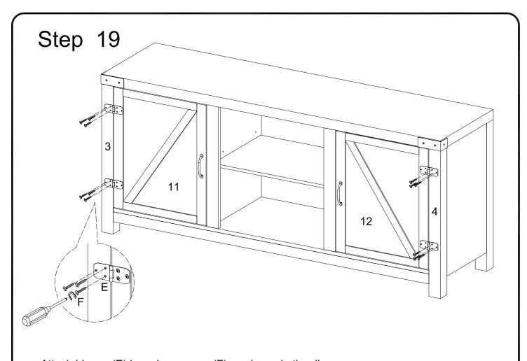
Attach hinges (E) by using screws (F) as shown in the diagram.
