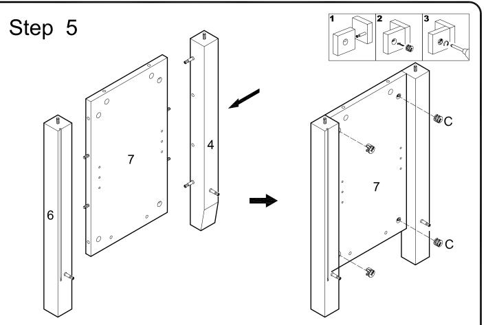
Attach parts (4) and (6) to the other part (7), and then insert cam locks (C) to the fully assembled part (7).
