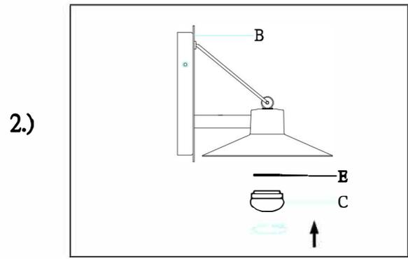
**Step 2:** Put the rubber washer (E) on the glass and then lock until tight.
