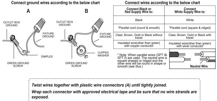
Carefully tuck all wires into the outlet box.
