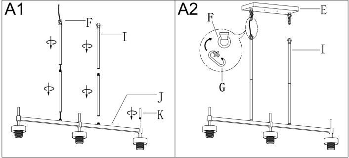
Step A1 » 1) Carefully pass the fixture wires through one side of loop (F) and tubes (I).
