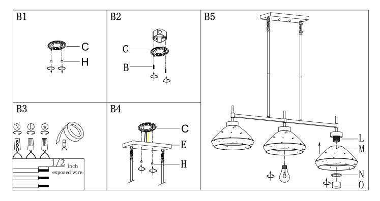
Step B1 » Unscrew knob nuts (H) from mounting plate (C).
