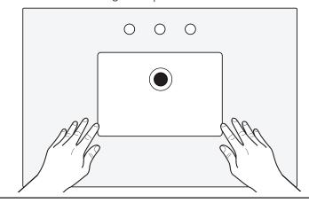
11. If you are installing a wood back-splash (available on specific models), place a generous amount of silicone sealant on the back of it and press it into place against your bathroom wall. Fill any gaps that are left with silicone sealant. Wipe away any excess sealant with a damp cloth.
