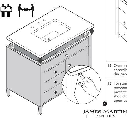
**10.** Once positioned, press firmly into place. Wipe away any excess sealant using a damp cloth.
