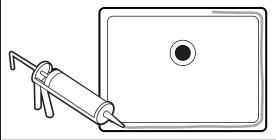
5. Carefully lift and turn the sink over on the countertop, positioning it within your marked outline, ensuring again that the overflow is opposite from the faucet holes. Once positioned, press firmly in place.
