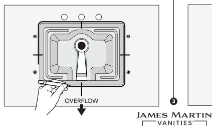
**4.** Carefully lift the sink from the countertop and place it on a soft surface, bowl side down. Apply a bead of silicone sealant around the top edge of the sink rim.
