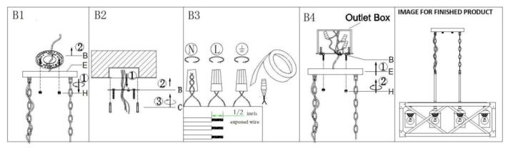
STEP B1: Unscrew the ball knobs (H) from canopy (E) then gently remove the mounting plate assembly (B)
