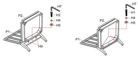
Step 2. Attach the left arm with leg (P3) and the right arm with leg (P4) to the seat frame (P2) and the chair back (P1) as shown below.
