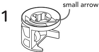
This is a Minifix cam. It has a little arrow on its upper surface.
