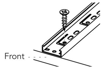
Take the bigger part of the slide and place it over the panel. The plastic stop should go towards the back.
