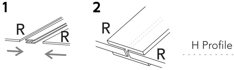
Slide the back panels inside the grooves.
