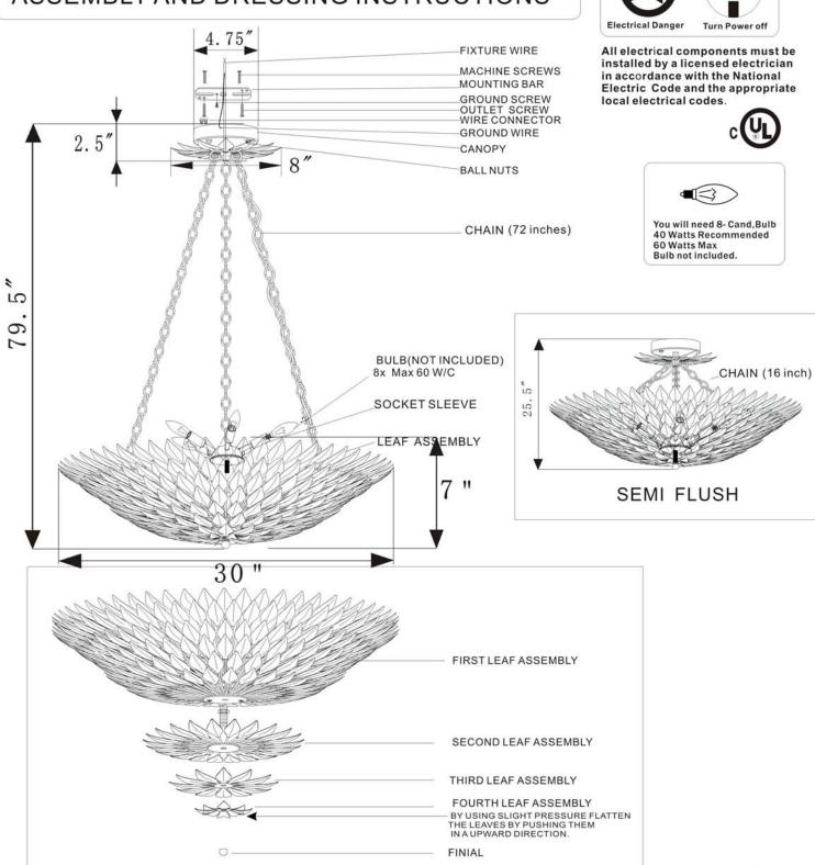
NOTICE: FOR REPLACING THE BULB, PLEASE UNSCREW THE LEAF ASSEMBLY AS SHOWN ABOVE
