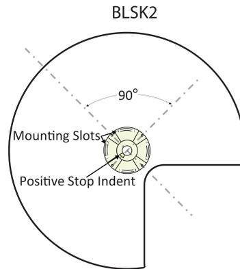
Turning a shelf upside down, position the Shelf Hub so that the positive stop indent is pointing to the left at 90 degrees from kidney cutout as pictured. Attach with four (4) - #6 x 1/2" Pan Head Phillips Wood Screws in the center of the mounting slots as shown. Turning shelf back over push the Shelf Collar into the top of the shelf until flush. Repeat with second shelf.
