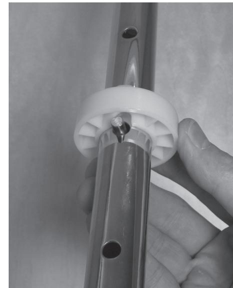
Raise upper shelf and Shelf Support to desired height and press steel pin through the closest hole in the pole. Lower the Shelf Support aligning the pin with the notches as shown. If Shelf kidney is misaligned to door opening, loosen screws in the Shelf Hub, position shelf and retighten screws.
