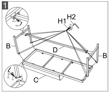
Step 1: Attach 2\*legs (B) \*\*The side with a screw hole is facing inward\*\*to assembled top (C) and connecting bar (D). Use Allen key (H2) to lock with 12\*Allen bolts (H1), as picture.
