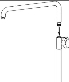
Assemble the overhead shower arm into the shower column. Ensure it is fully seated. Install 1 of the set screws into the shower column and tighten.
