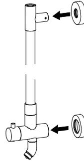
Assemble the upper escutcheon and lower escutcheon onto the upper and lower post of the shower column, respectively.
