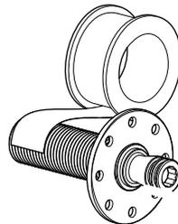
Apply plumbers tape to threaded end on the inlet fitting.
