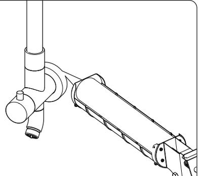
Slide the upper and lower escutcheons back against the finished wall. Apply silicone sealant to the rear lip of the upper and lower escutcheons.
