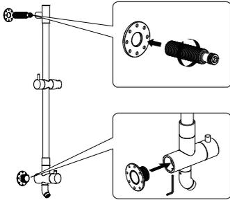
Hand tighten upper mounting flange onto inlet fitting.
