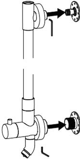
Install the shower column onto the inlet fitting and lower mounting post. Then use the hexagonal wrench to tighten the hexagonal socket screw set.
