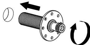
Thread the inlet fitting into the built-in pipe outlet and hand tighten.
