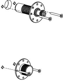
Thread the inlet fitting into the built-in pipe outlet and tighten using a smooth jawed wrench.
