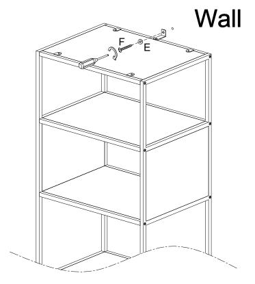
Secure furniture to anchor (G) in wall using washer (E) and screw (F) with a screwdriver.
