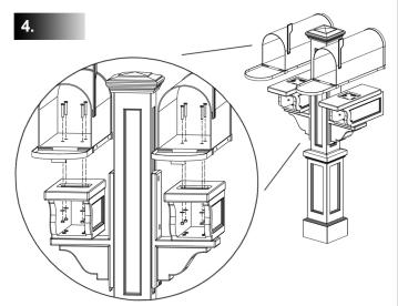
Pre-drill 4 holes with a 3/8" drill bit through the mailbox and paper holder arm as shown above. Using a nut, bolt, and washer combination secure the mailbox to the arm and tighten. 2" bolts are recommended (mailbox and mailbox mounting hardware not included).
