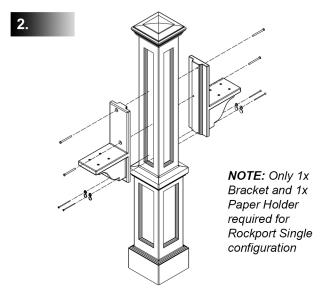
Fasten the two brackets (part 3) to the post as illustrated above. Use two 3" lag bolts (part 4) in the top 2 holes on each bracket and two 3" screws (part 5) on the bottom. Plastic snap caps (part 6) are provided to cover the screw heads.
