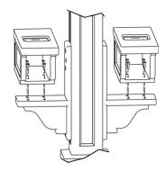
For each Newspaper Holder Insert 4 truss screws (part 7) through the drilled holes and into the nuts already molded in place on the brackets. A short handled screw driver is recommended to tighten the truss screws inside the newspaper holder.
