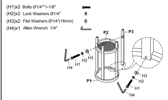
Step 4. Securely tighten all bolts with Allen wrench(H4), turn the assembled table to an upright position, Assembly is complete.
