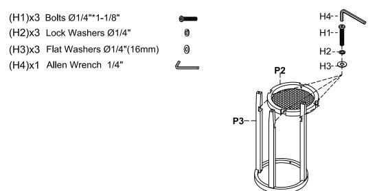
Step 3. Attach the fourth leg (P3) to the assembled shelf (P2) and table top (P1) as shown below.
