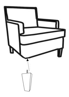
Step 1:Take out two front feet and two back feet from the carton and put into the screw holes underneath the base and screw tight to the right angel.
