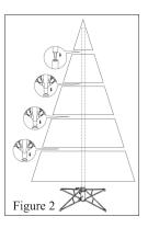
Step 3 Unfold the branches one-by-one beginning with the lowest.
