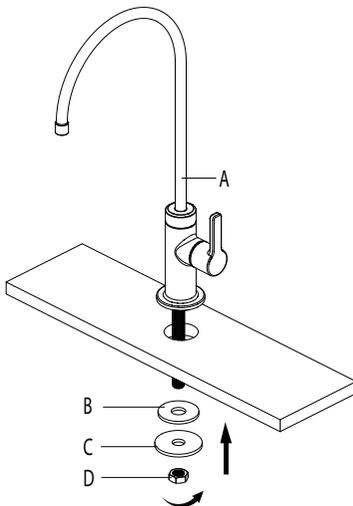
Place the faucet assembly (A) through the selected hole in the sink or countertop. On the underside of the sink or countertop, slide the rubber washer (B) and metal washer (C) onto the stud. Thread the mounting nut (D) onto the stud, and tighten securely using your wrench.
