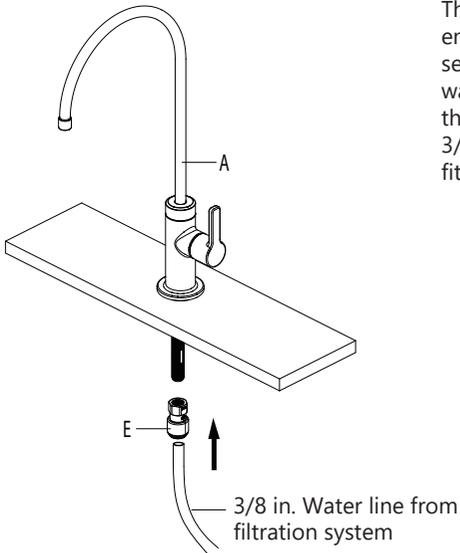
Thread the quick connect adaptor (E) onto the end of the faucet assembly (A) stud, and tighten securely using a wrench. Connect the 3/8 in. water line from the filtration system by pushing the line into the connector (E). Pull down on the 3/8 in. line slightly to ensure the quick connect fitting has engaged.
