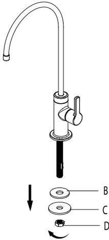
Remove the rubber washer (B), metal washer (C), and mounting nut (D) from the end of the stud.
