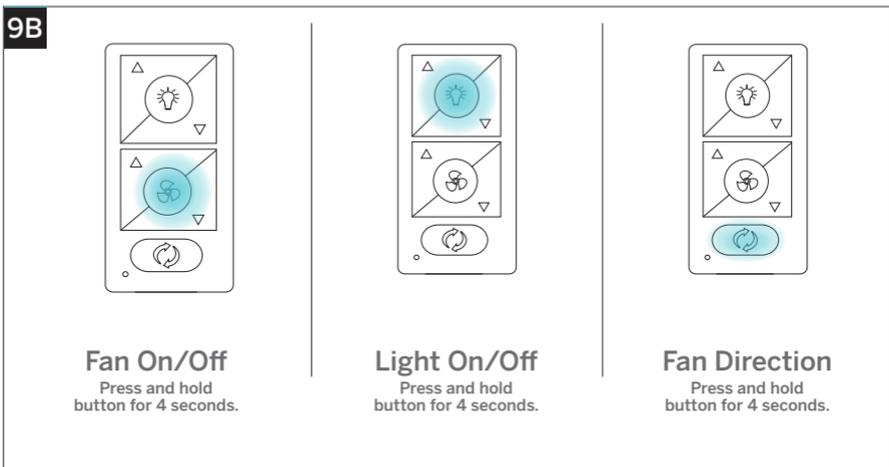
**Fan On/Off:** Press and hold button for 4 seconds. The LED on the remote will flash green and all connected fans will beep to indicate the message has been received. All fans will turn off. This will bring all fans controlled by the remote into sync.
