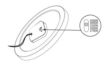
3 Carefully tuck the wires into the J-Box, align the spring clips on the fixture to the bracket holes and push the fixture flush to the ceiling, snapping the clips into the bracket.
