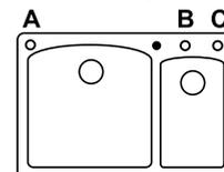
Note: Distance between B & C holes is approx. 5" on center, because of clip location.
