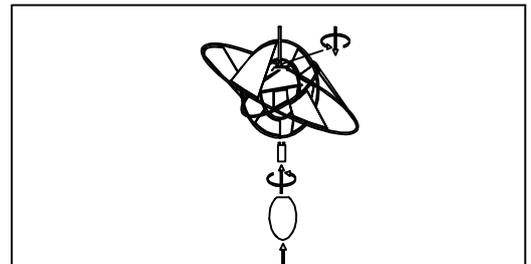
Step.3: Pack the GU24 LED light source(G), pack glass(H) to twist good glass(H) of tight iron piece lock.
