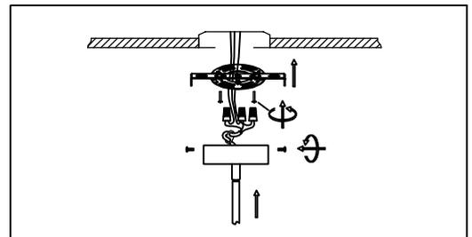
Step.2: Use screw(D) hang plank(C) to install well, use spring coil Luo the type connect the line head(E) has the power cable connected and use screw(F) light body gearing to hang top in the plank
