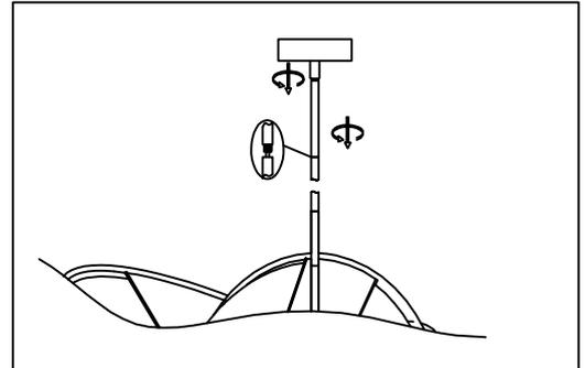
Step.1: Link the pipe line(A) to the light body, absorb a dish to pack with ten thousand toward the head(B) in the pipe line
