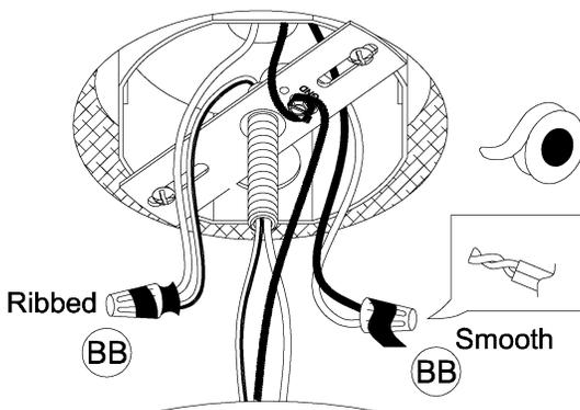
5. Strip 3/8" of insulation from the electrical wire ends. Using wire nuts (BB), connect RIBBED fixture wire to the WHITE supply wire from the outlet box; connect the SMOOTH fixture wire to the BLACK supply wire. Connect the fixture ground wire and supply ground wire using a wire nut or by fastening to the ground screw on the mounting plate. Push all wire connections into the outlet box.
