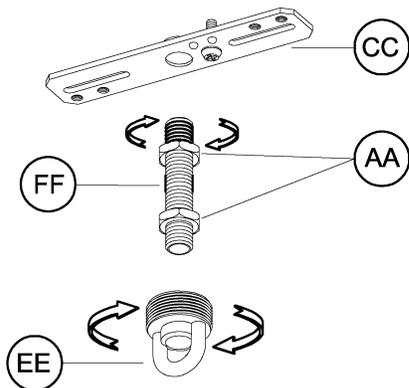
1. Screw threaded nipple (FF) into mounting plate (CC) several turns. Use one hex nut (AA) to secure parts tightly. Screw one hex nut (AA) and chain holder (EE) onto threaded nipple (FF). Tighten the hex nut against the top of the chain holder.
