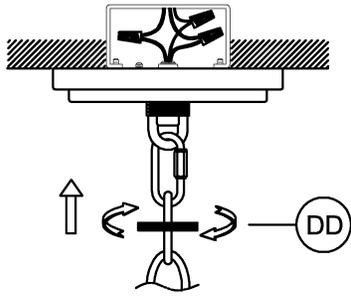
6. Tuck the wires into the outlet box and slip the canopy over the chain holder. Thread the screw collar (DD) onto the chain holder to secure the canopy tightly to the ceiling.
