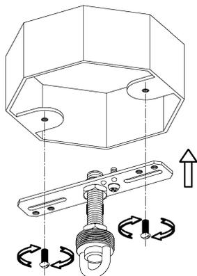
2. Attach assembled parts from step 1 onto outlet box using the mounting screws supplied with the outlet box (not included).
