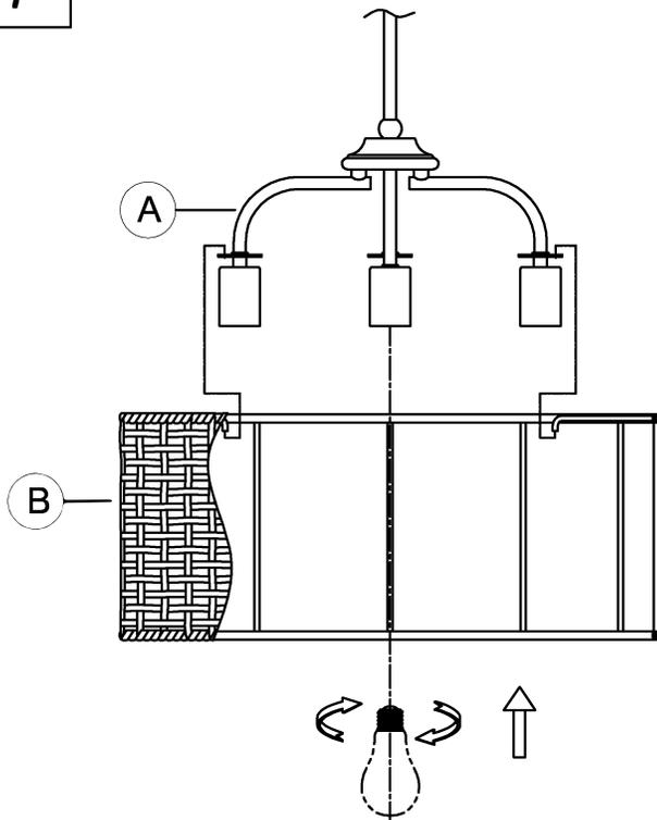
7. Place wicker shade (B) onto fixture (A). Screw lamps (not included) into fixture socket. Use 60-watt MAX incandescent medium base lamp, SBCFL or SBLED.
