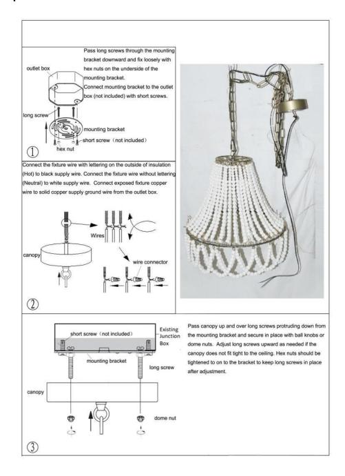
NOTE: Wire with lettering or specification shown on the outside is HOT and should be connected to the Black or Red supply wire. Fixture wire without lettering is the Neutral wire and should be connected to the White supply wire. Copper ground wire from the fixture should be connected to the copper supply wire.
