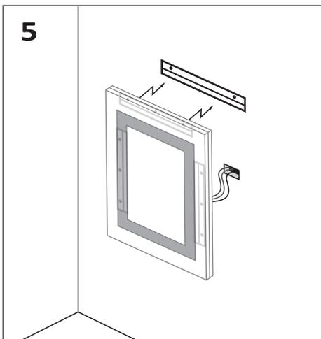
Line up the bracket of the mirror with wall bracket and slide the mirror down
