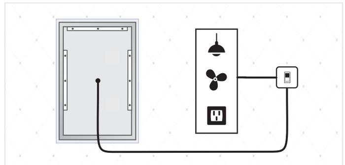
*Install optional outside switch to control the defogger
