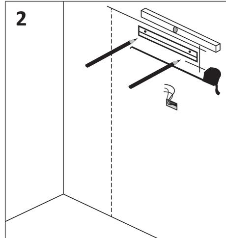
Mark hole positions on the wall ready for drilling
