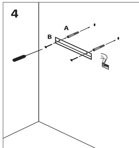
Insert anchors into predrilled holes and fix the mounting bracket to the wall
