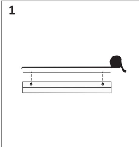
Measure distance between holes for the mounting bracket installation
